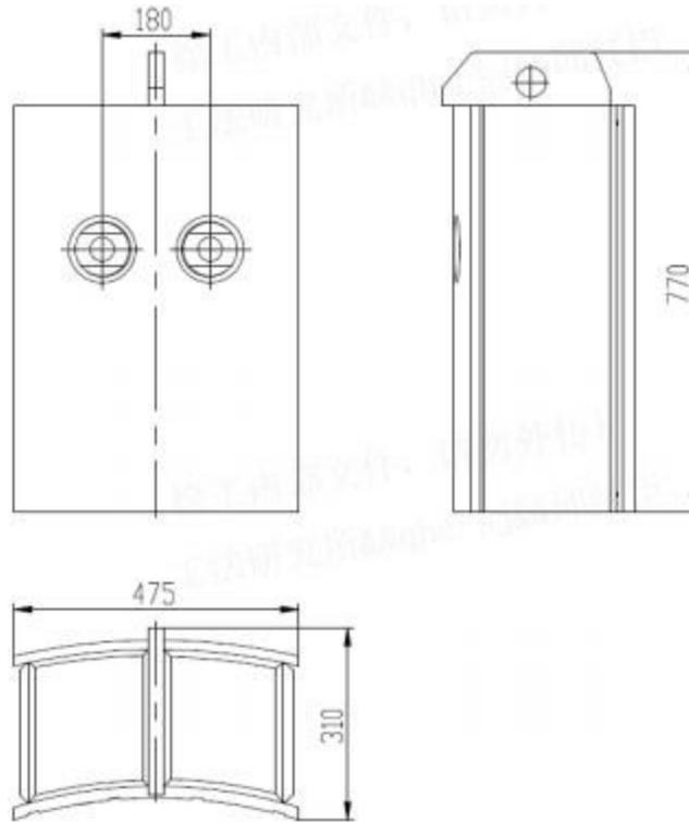
The main variable diameter block  $\phi 2100\text{mm}$  variable  $\phi 1600\text{mm}$  total 8 pieces, single weight 200Kg
