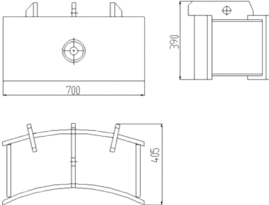
Side variable diameter block  $\phi 2100\text{mm}$  variable  $\phi 1200\text{mm}$  a total of 8 pieces, a single weight of 205 kg.
